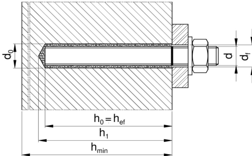
**Anchor application in hollow/perforated masonry with nylon sleeve (brick n°2 according to Annex B9)**
