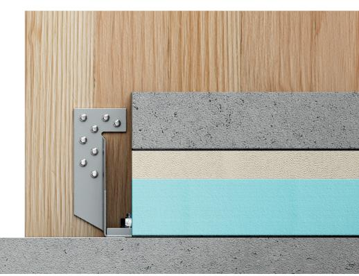
At 140 mm high, HDCLT is completely concealed once the floor membranes, insulation and acoustic layers are in place.
