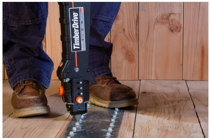
Precision-placement nosepiece for steel-to-wood fastening.
