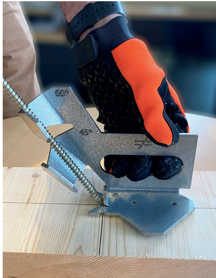
Example of skewed installation - GSCREW4560-R
