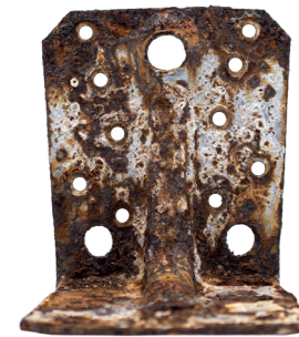
Galvanised Steel Z275 Coated Connector Most of the connector is completely rusted.
