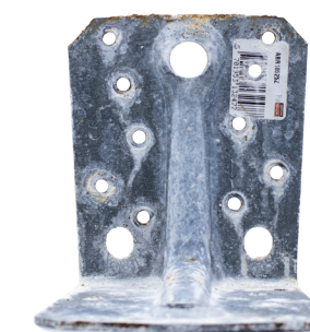
ZPRO Coated Connector Rust forming on the edges becomes coated with protective magnesium deposits.
