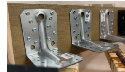
Comparison after 4,000 hours in salt spray testing chamber
