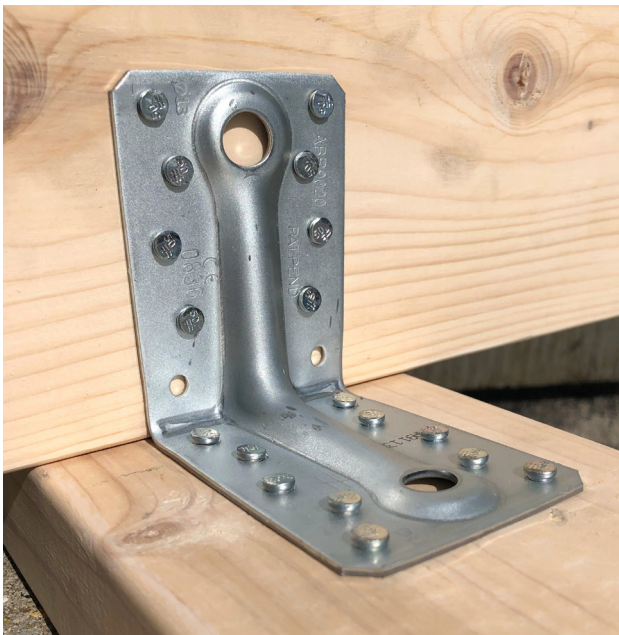
ABR9020 reinforced angle bracket installed with CNA4.0X50 connector nails.
